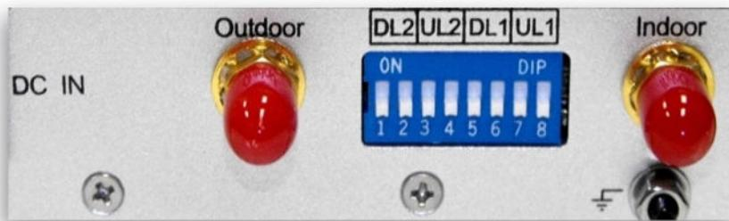
Depending on the frequency band of your repeater, it will determine the dip switches you will need to adjust and the corresponding LED that will show the status of the adjustments made.
